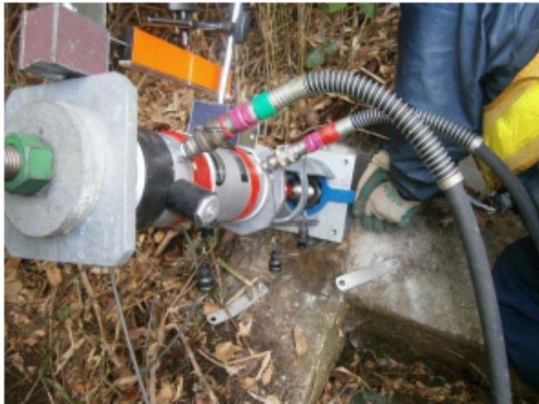
(a) The Lift off test performed by the hydraulic jack
