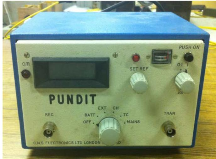
図4.2.3 PUNDIT (CNS Electronics製)
