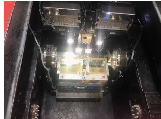
Preparation of embankment model in a soil chamber subjected to 50g acceleration
